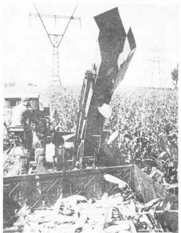
A maize harvester produced by the Agricultural Mechanization Research Institute in Heilongjiang Province.
