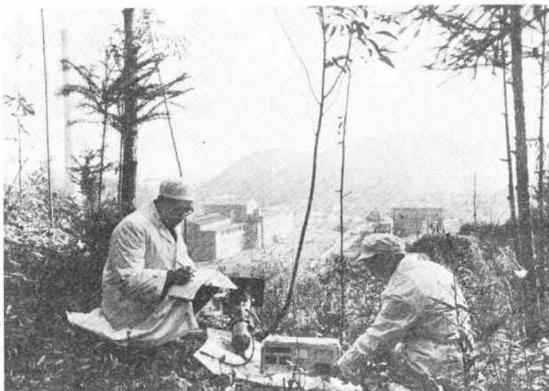
Environmental specialists taking air samples and monitoring the atmospheric effects of a high-flux reactor.
