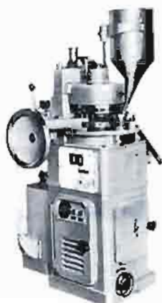
Rotary Tablet Press Model ZP-19
