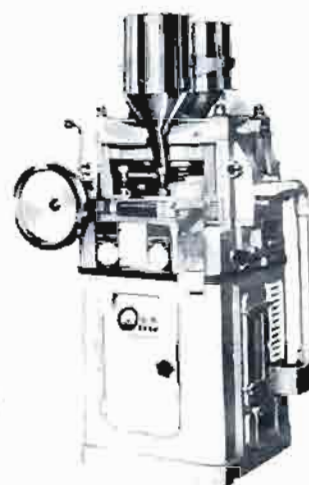
Rotary Tablet Press Model ZP-33
