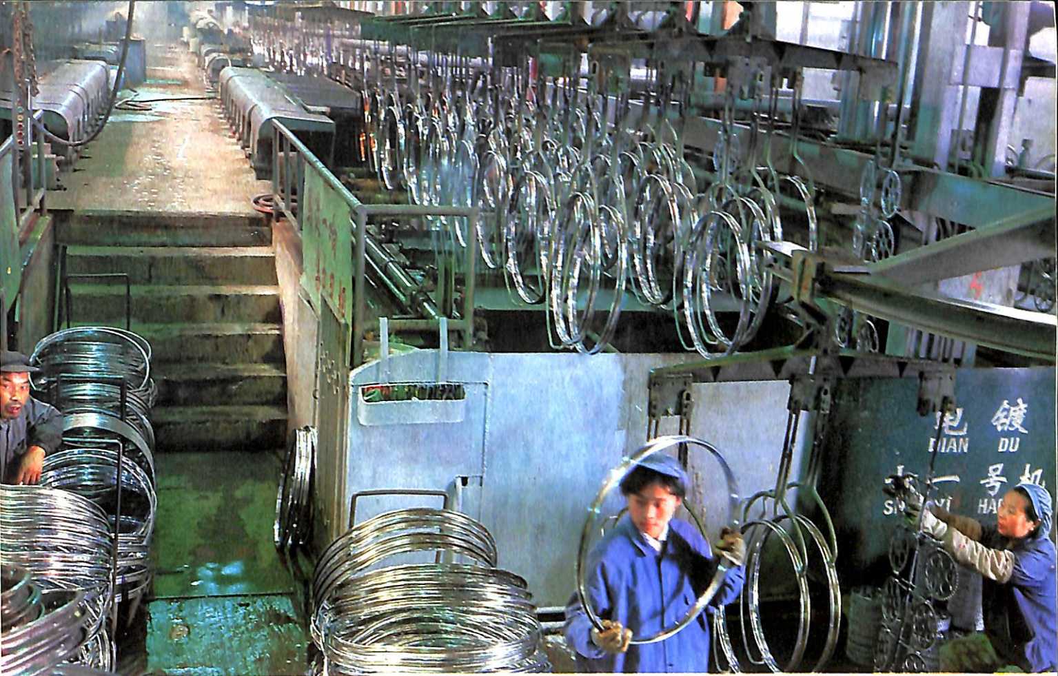
Automatic production line for electroplating in a Shanghai Bicycle Plant.
