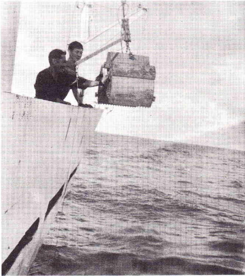
Workers on the Xiangyanghong 09 use a redesigned silt collector to get samples from the bottom of the sea. Song Wenbo
