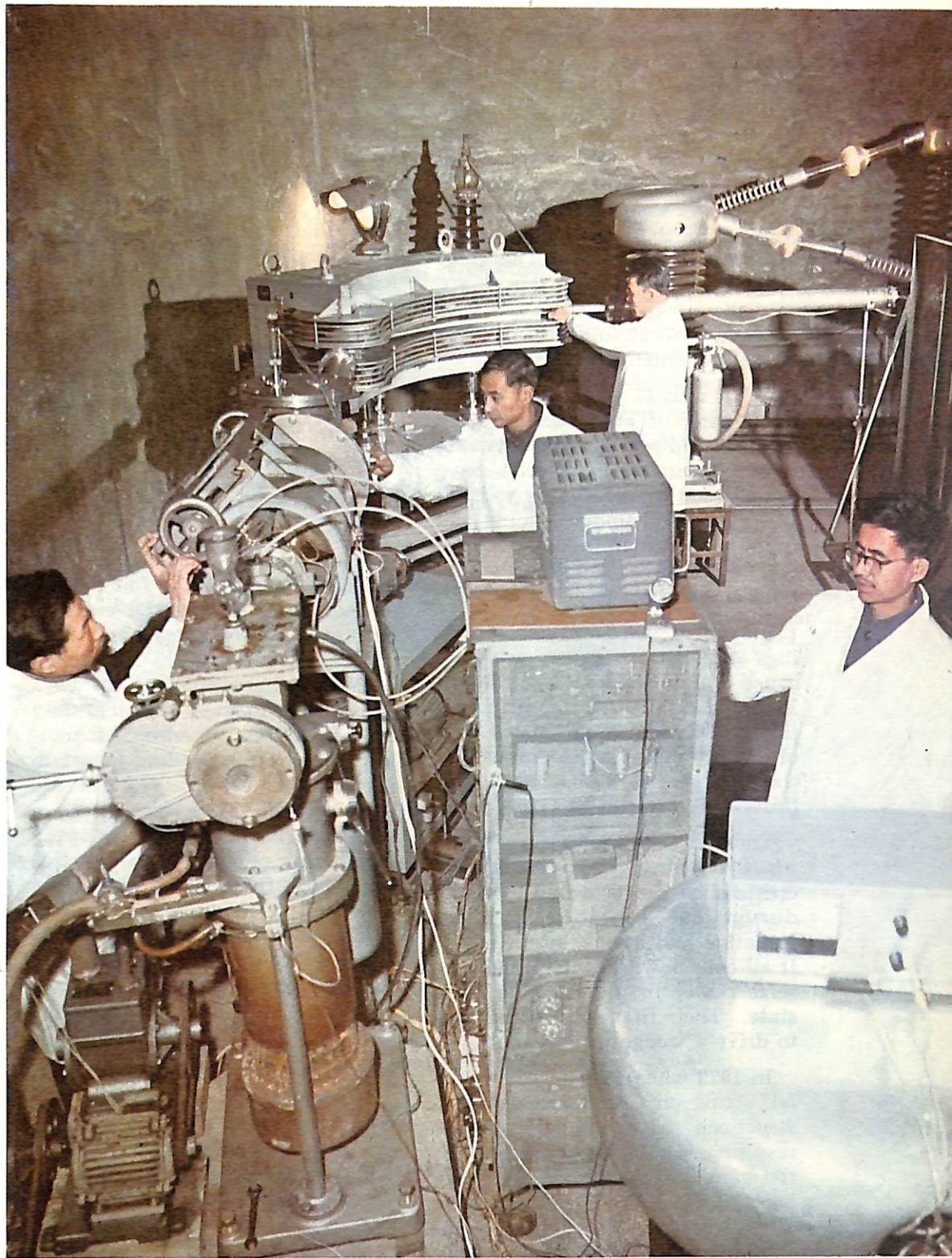
A 400-kilovolt heavy ion injector, first of its kind made in China, a research project of the nuclear physics faculty of Peking Teacher's University, made with the help of related factories and completed in 1977.
