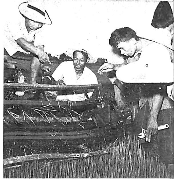
The Party secretary and members of the commune discuss improvements on a new machine for pulling up rice seedlings for transplanting.
