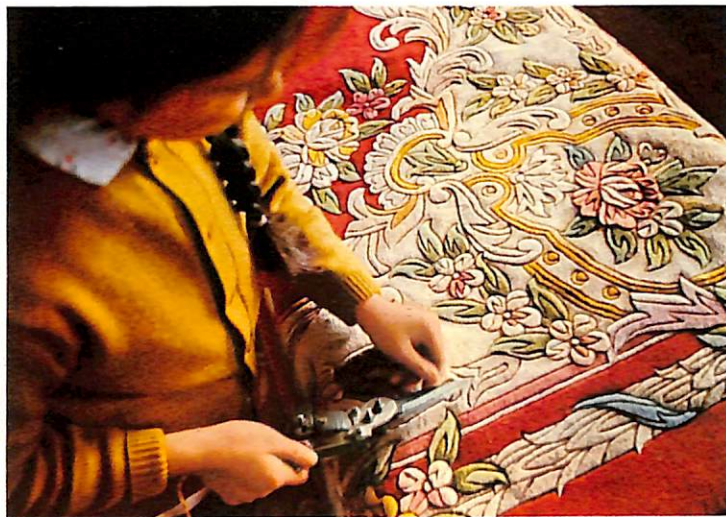
Clipping the pile
