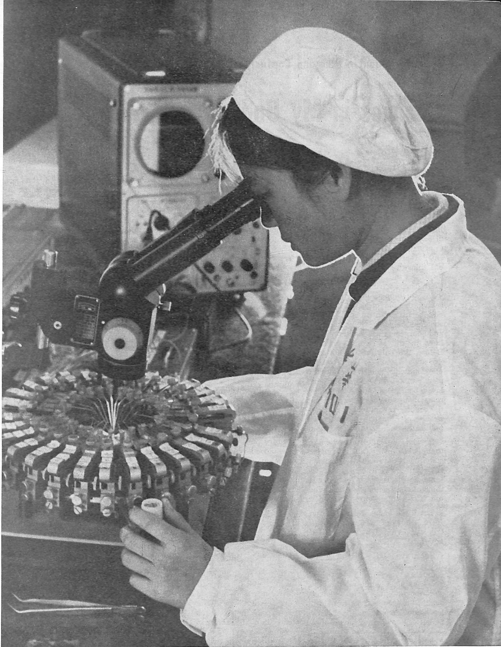
A worker in the semiconductor shop of Tsinghua University making intermediate tests on MOS integrated circuits.
