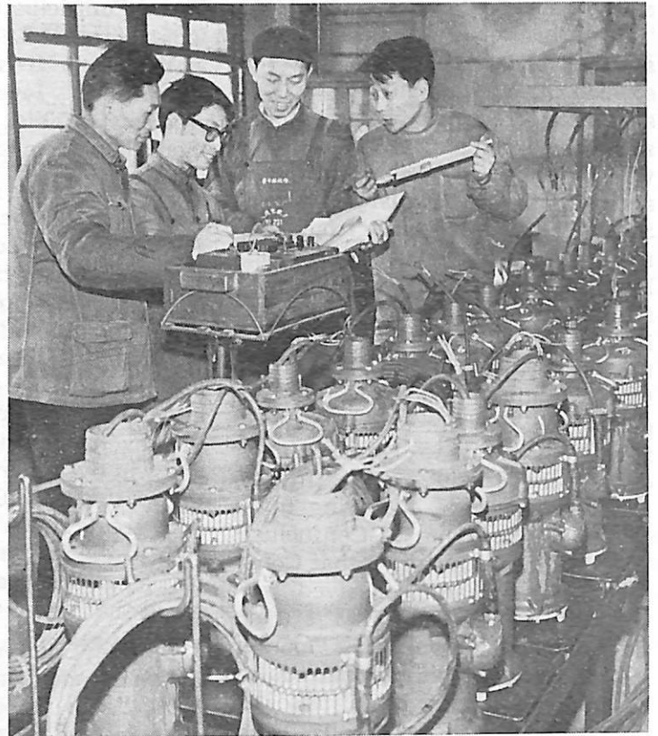
The Shanghai People's Electrical Machinery Plant testing oil-immersed submersible pumps.
