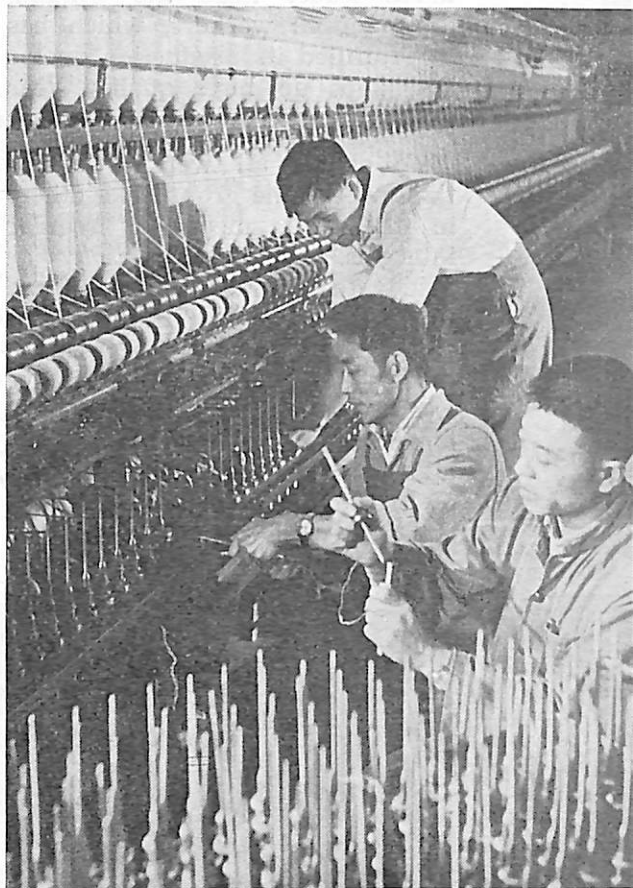
Installing the new high-speed spindles.
