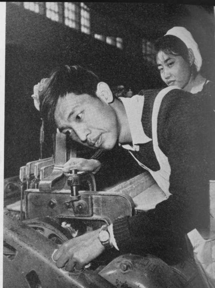
Chou So-kuei listening to the sound and "feeling the pulse" of a loom to check its running.
