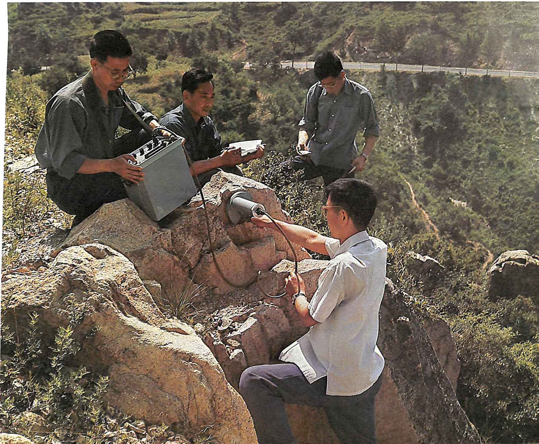
Elementary analysis conducted by geologists in the open by using a radioactive isotope X-ray fluorescence analyser.
