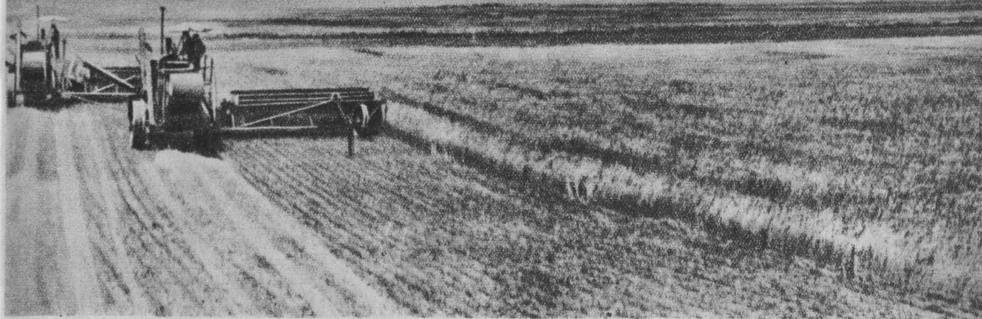
Each No. 6 Stalin combine-harvester reaps and threshes four and a quarter acres an hour
