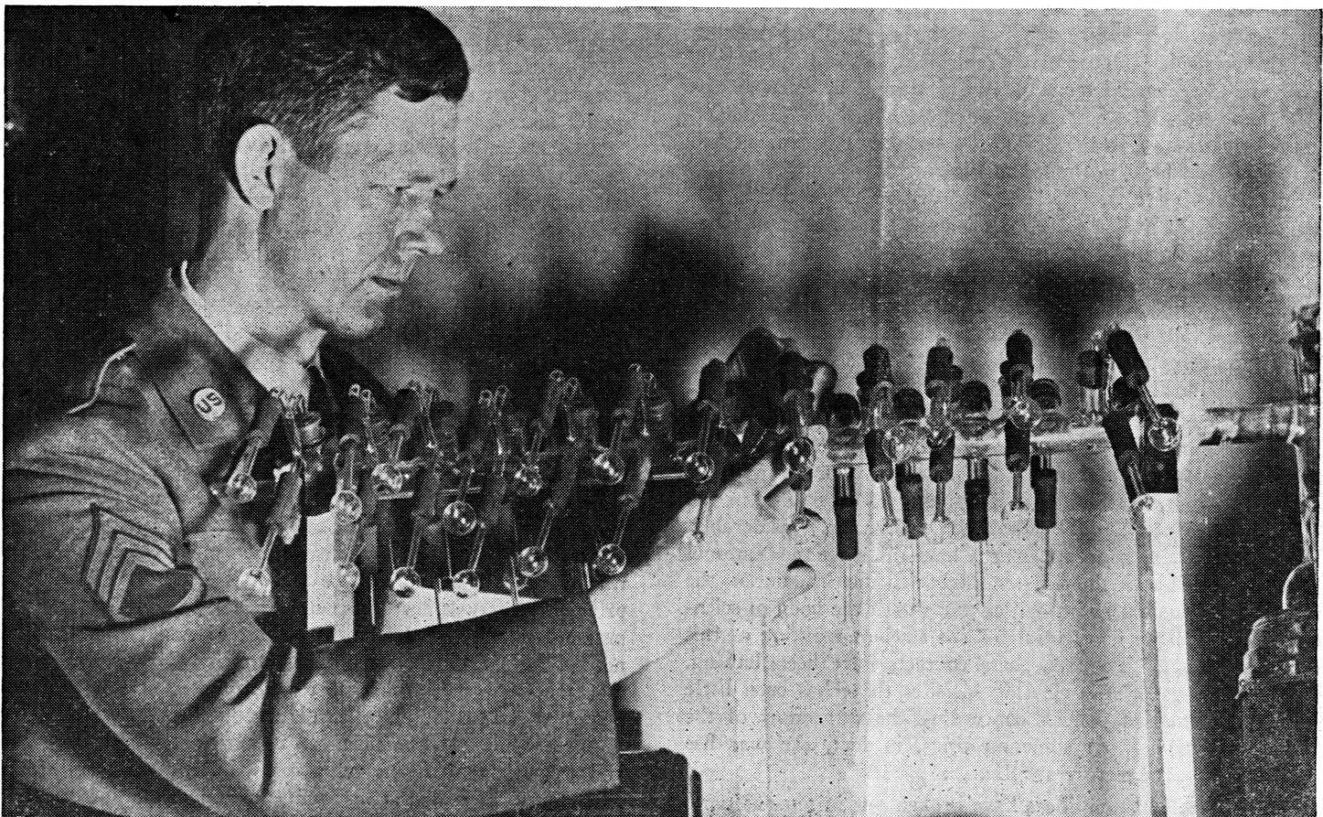
A scientist in the Army Medical School's Division of Bacteriology preserves bacterial cultures and viruses by freezing and drying in vacuum.
