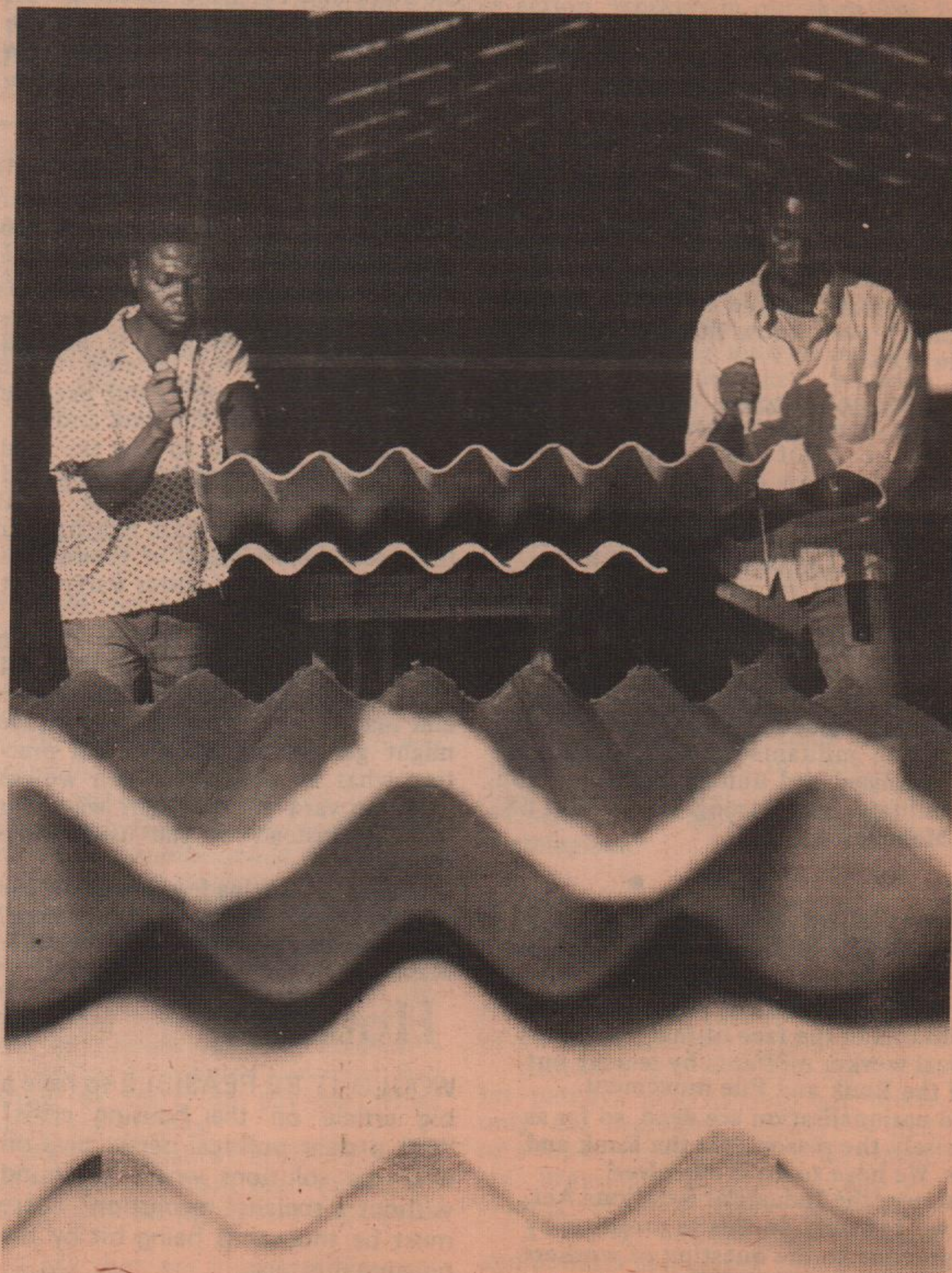
Nigerian workers cutting asbestos-cement sheeting without any protection from the asbestos dust. The photograph proudly appears in Turner and Newall's 1973 publicity brochure.
