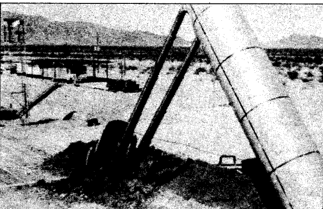
AN MX missile goes into firing position from its underground track
