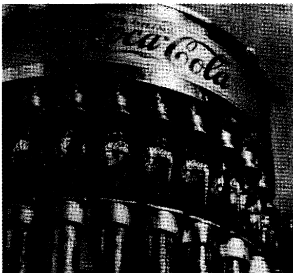
Pipes from storage tanks carry syrup to the Syruper which dispenses the right amount into each bottle.
